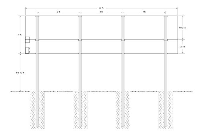
Once you have verified the positions of the posts and the size of the footings, you are ready to dig your holes, pour your concrete, and set your posts. There are several techniques for ensuring proper alignment of the posts. Typically installers will construct a temporary wooden support frame to hold each post in place while the concrete sets. Having plumb posts in the proper position is the key to a smooth mechanical installation.
