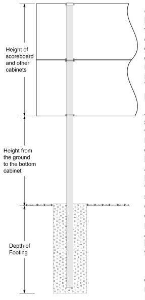
The length of your posts is determined by the configuration of your scoreboard display, its height above the ground, and the depth of your footings. Footing size is also related to the cabinet height and configuration. To some degree, the depth of the footings will be determined by the equipment available to the installer. In general, a smaller diameter hole needs to go deeper than a larger diameter hole. The trick is to create footings hefty enough to provide stability for the sign structure.
